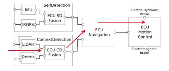
$P[S_k] := \lambda_{LIDAR} \lambda_{Camera} + P[DisfECU_{CD}] \\ + \lambda_{IMU} \lambda_{RGPS} + P[DisfECU_{SD}] \\ + P[DisfECU_{Navigation}] + \lambda_{MotionControl}.$
