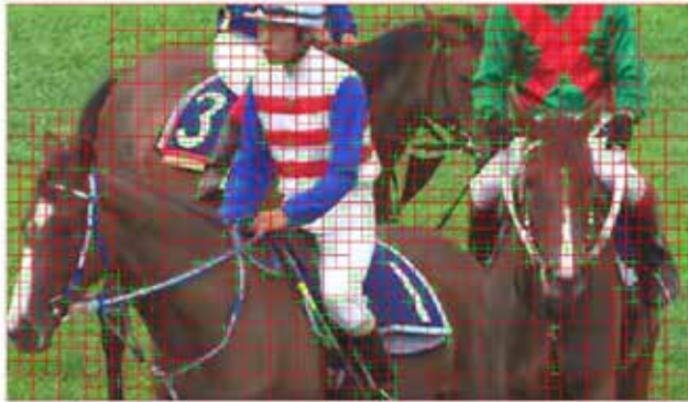
Fig. 1: Example of frame splitting into CUs (red) and PUs (green) based on the HEVC quadtree structure, RaceHorses .
